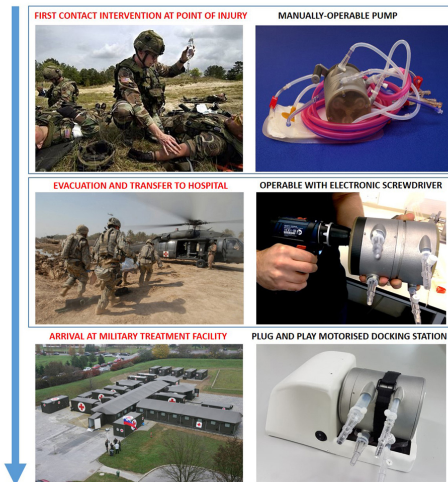
Figure 7 The technology was designed to treat—through autotransfusion and cell concentration—the casualty throughout the entire journey from the point of injury, during the evacuation and transfer to hospital stage and ultimately at arrival at a military treatment hospital.
